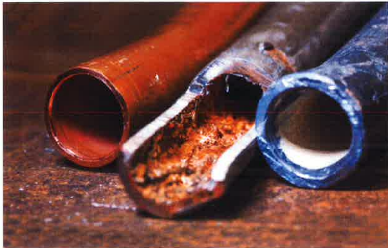
Pipes pictured (L to R) copper, untreated lead and lead treated with phosphates
